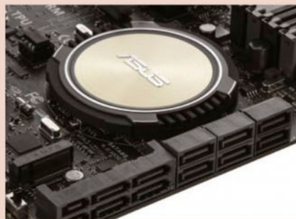
▲ In addition to SATA 6gbps ports, Z97 also now supports SATA Express, enabling you to use up to two lanes of PCI-E 2
