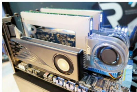
Two Revodrive 350s configured as RAID 0 and with extra cooling.
