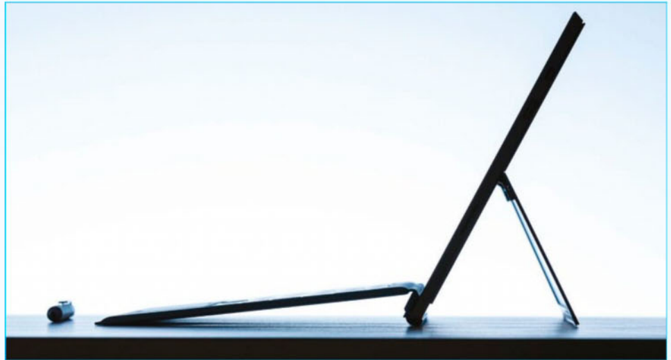
▲ The Surface Pen is thicker than the Surface Pro 3, and so can't be stowed neatly in the device
